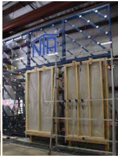
Air, Water, Structural Testing
